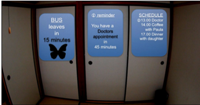
Fig. 24. Reminder and guidance concept in a bedroom environment, displayed on the closet surfaces. Reprinted from paper III
