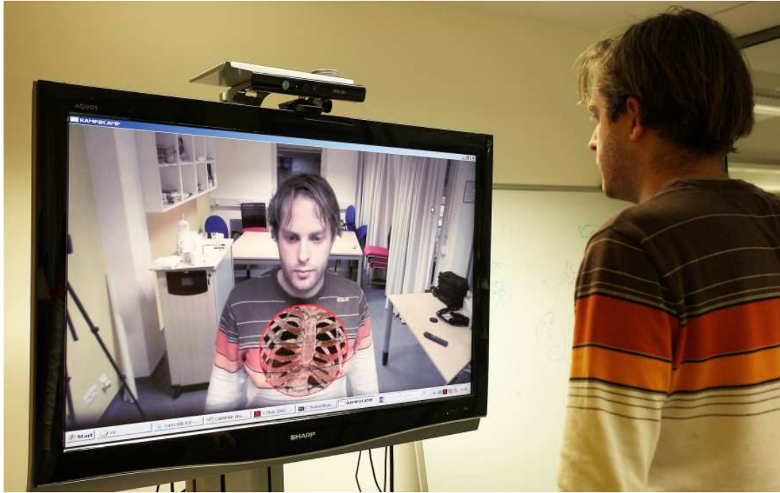
Figure 2.6: The miracle system [13], a mirror AR system that helps users learn about anatomy.
