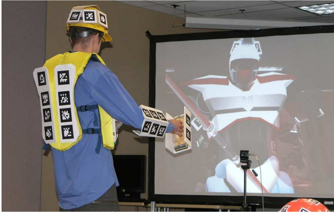
Figure 2.10: Fiala’s magic mirror system [31]. A user wearing AR markers is reflected and augmented virtually by the mirror.
