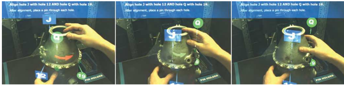
Figure 2.9: The AR instruction system proposed by Henderson and Feiner [40]. The AR arrows instruct the user on how to move in 3D space.
