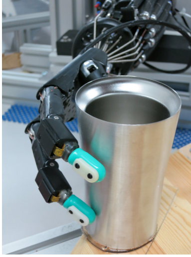
Figure 5.2. Tactile object recognition by a robot hand
