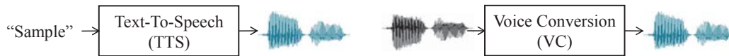
Figure 3. Speech synthesis techniques used in this thesis; Text-To-Speech (TTS) and Voice Conversion (VC). TTS and VC do not use the same input types, but they share in common certain internal processes.
