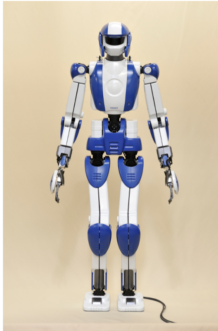
Figure 3.9: Humanoid robot HRP-4. This humanoid manufactured by Kawada Industries is 151 cm high, weights 39 kg, and has 34 DOF.
