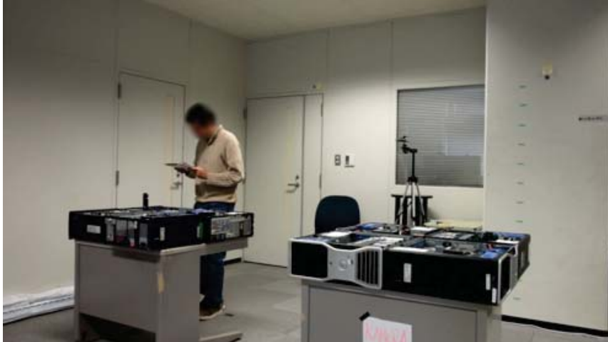
Figure 3.3. A test user conducting the machine inspection study. The machine is on top of a table and an omnidirectional camera is in the middle to capture participant's face for the gaze shift measurements.
