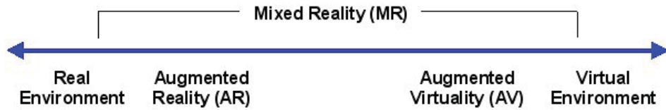
Figure 1.1. The reality-virtuality continuum. AR and AV form the mixed reality that contains both real and virtual elements. [52].
