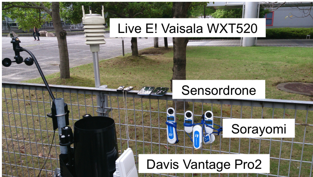
Figure 27: First measurement setup using different sensors
