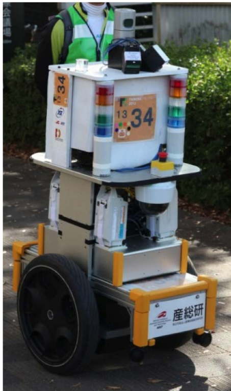
Fig. 35 A mobile robot “EMU” based on Segway RMP200ATV
