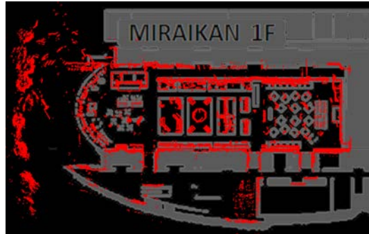
Fig. 42 Floor plan and maps generated by conventional method (in Miraikan 1F)
