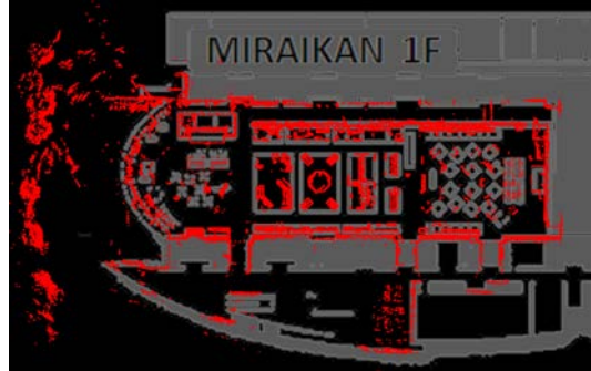
Fig. 41 Floor plan and maps generated by proposal method (in Miraikan 1F)
