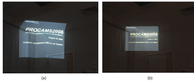
Figure 4.18. Example of an apparent plane projection onto an arbitrary curved surface by considering geometry information of the projection surface from [91] (a) Without geometrical consideration (b) With geometrical consideration
