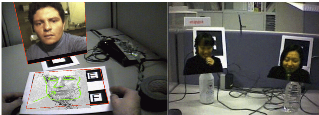
Figure 1.3. Live images of remote users are rendered on fiducial markers for a teleconference session [9].
