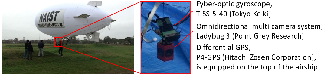
Figure 3.1. Unmanned airship and mounted sensors
