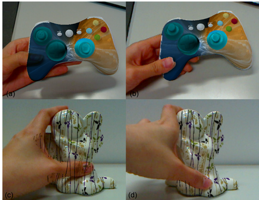
Figure 6.3. Texture occlusion on the (a) game controller prototype and the (c) angel figurine. On the left, the object texture is rendered on the user's hand. On the right, correct display of the texture by removing it from the occluded parts.
