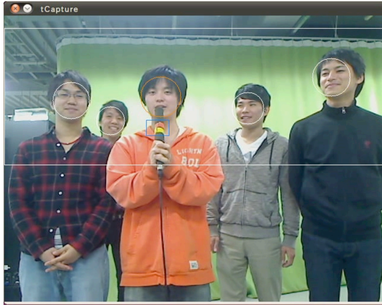
Figure 5.4: An example of the image processing, where circles indicate the results of face detection and the blue square indicates the result of color extraction for microphone detection
