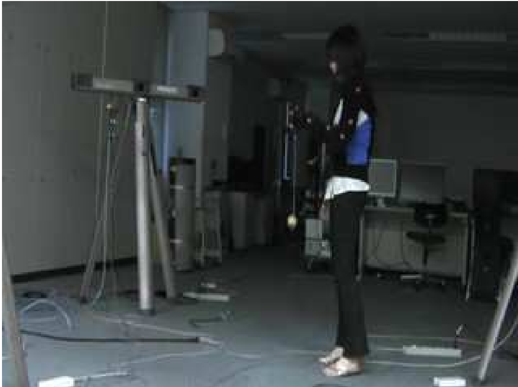
Figure 4.2: Experiment setup. The upper arm of human and kendama cup and ball motions are measured by using optical motion capture.
