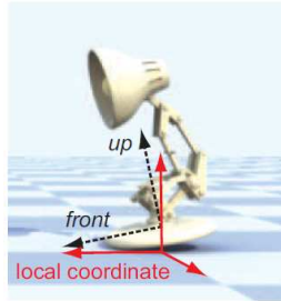
Figure 2.3: The local coordinate frame (shown in solid, red line) for representing the feature point positions.
