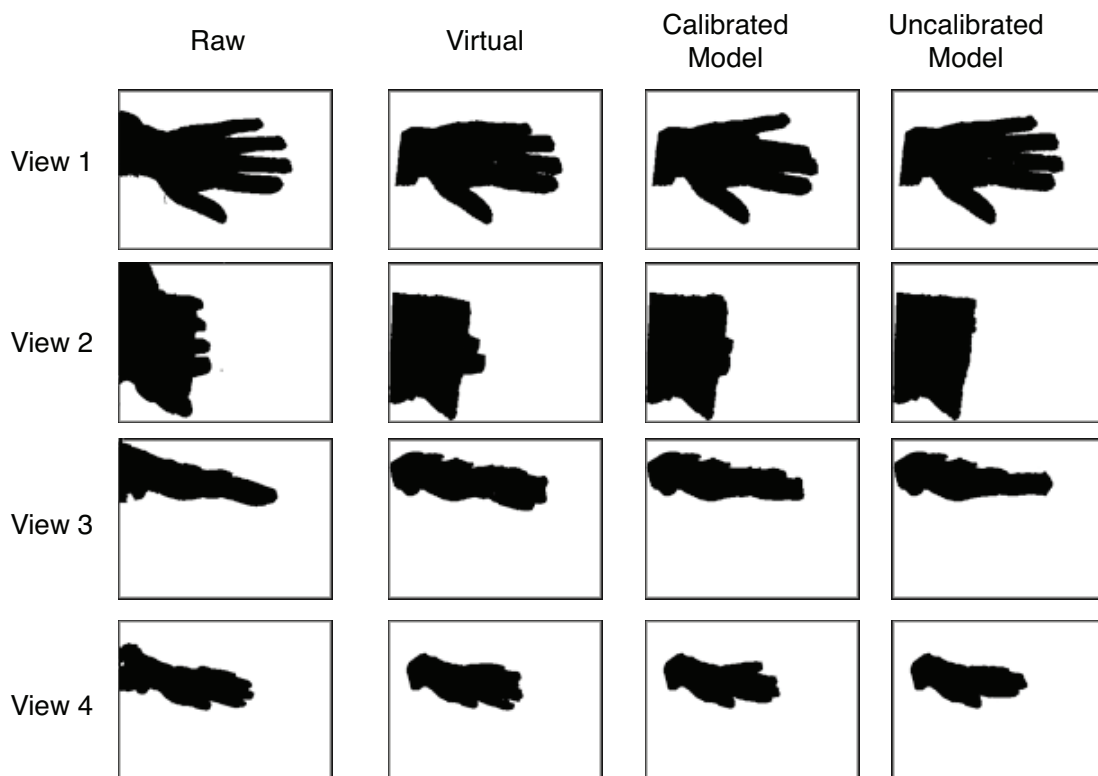
Figure 3.27: Comparison of silhouette area ratio for the virtually generated cyberglove motion, pose estimation using calibrated model, and using uncalibrated model for Point 2 of Figure 3.25. The uncalibrated model shape is rendered using the calibrated model to minimize bias in comparison.
