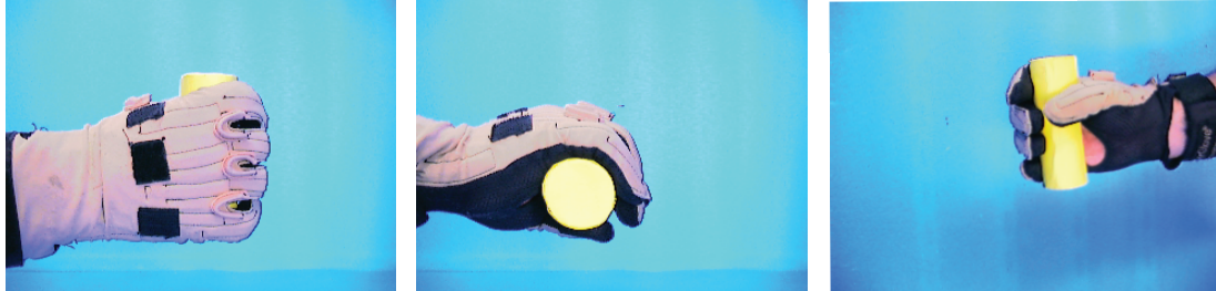
Test Pose 1: Grasping a cylinder.
