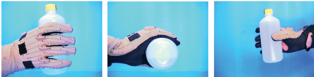
Test Pose 2: Grasping a cylindrical pet bottle.
