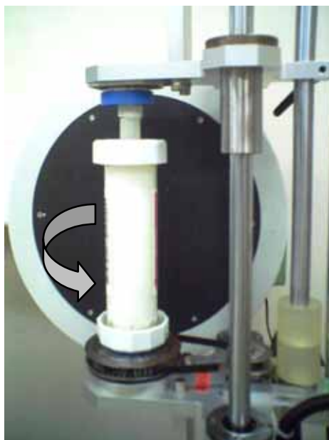
Fig. 30 Rotating table and a column setting. Rotation speed: 3 rot. / min
