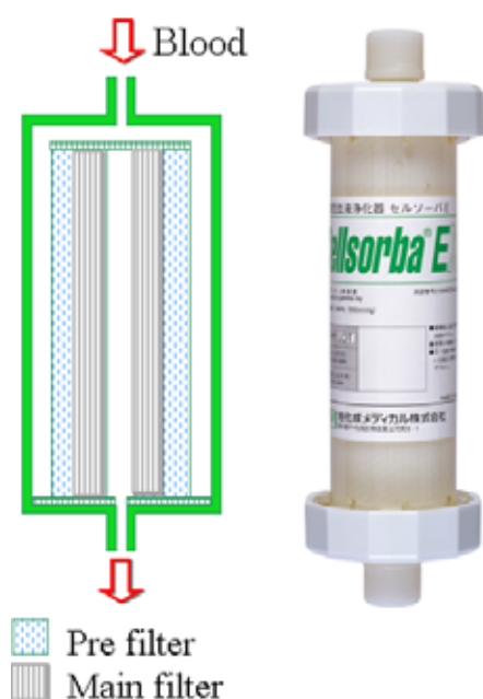
Fig. 24 Structure of leukocyte removal column.
