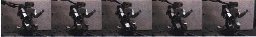
Figure 4.9: An acquired whole-body punching movement on real hardware system. The snapshots are corresponding in 0.0 sec, 1.0 sec, 1.5 sec, 1.8 sec and 2.0 sec, respectively.
