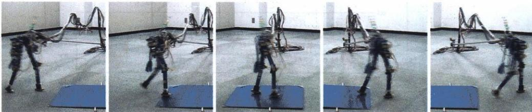
Figure 3.9: Example of an environmental change. Walking pattern on a seesaw-like metal sheet
