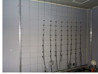
(b) Plain type microphone array
