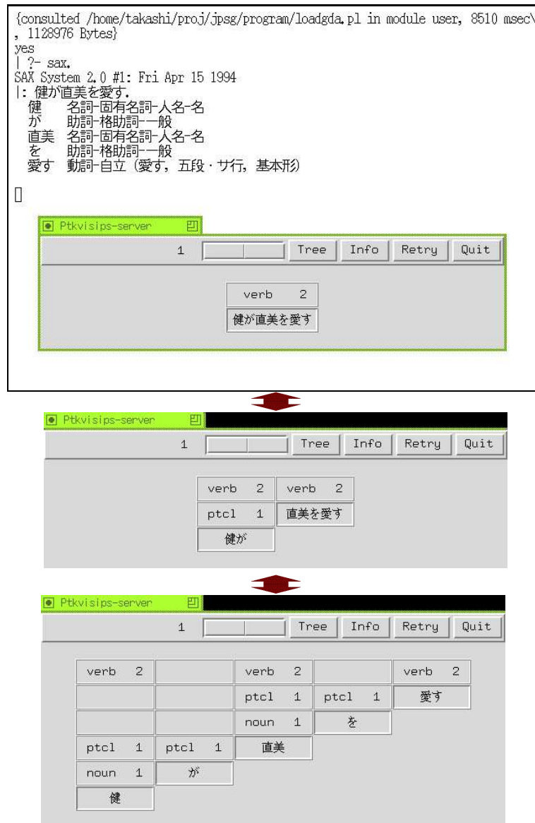
Figure 3.6: Folding and Unfolding the CKY Table
