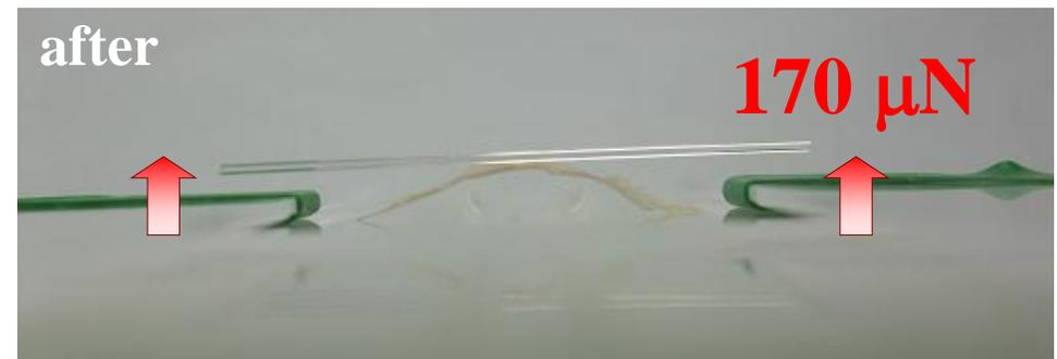
➔ Polymer film of poly(3HCA) lifted up the weight of glass tube to produce mechanical force (**170  $\mu\text{N}$** ).
