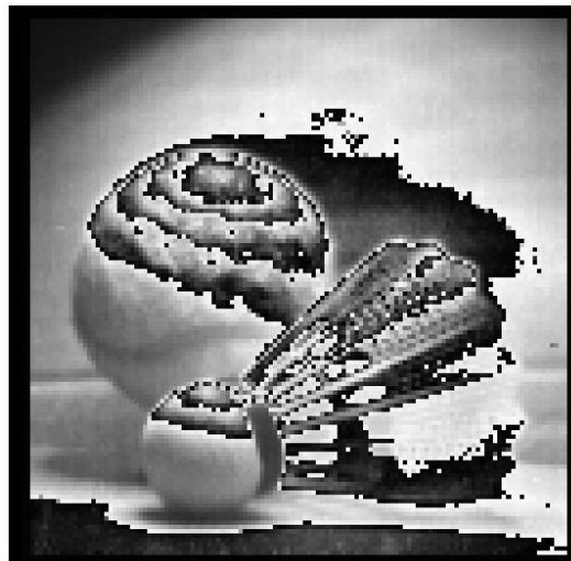
Figure 52 An image taken by the self-reset image sensor using a lens to show the resetting boundary along the surface with different light intensity.
