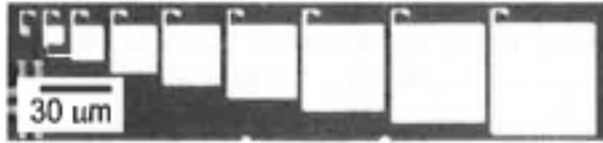
Figure 3.4 Optical micrograph of mesa patterns defined in amorphous Ge for grain boundary filtration.
