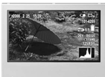
2.7-inch TFT LCD Module [NL9654HLO6-01J]
