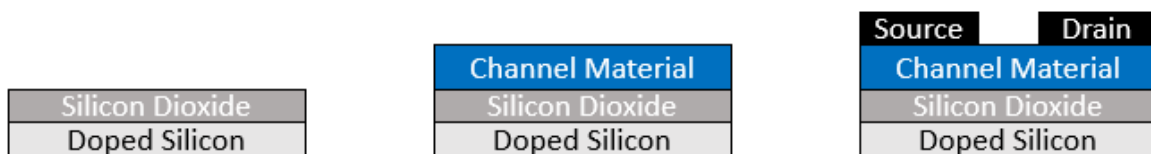
Figure 1.5 Simplified version of the TFT device fabrication process.
